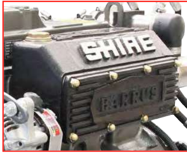
Water cooled manifold
