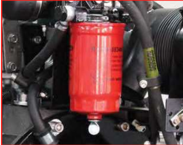
Fuel filter with water drain separator
