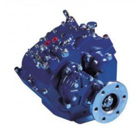
The hydraulic operating system functions on normal lubricating oil of the same viscosity as that used in the engine, avoiding the need to use automatic transmission fluid, and ensures rapid response to movements of the operating lever for good boat handling. The operating lever has a positive neutral detent and is suitable for use with proprietary single lever remote control operating systems.
