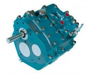
The gearcase is constructed of high grade cast iron, internally ribbed for rigidity and strength, and consists of two separate halves to facilitate servicing, the oil pump and hydraulic control valves being externally mounted for easy accessibility.
